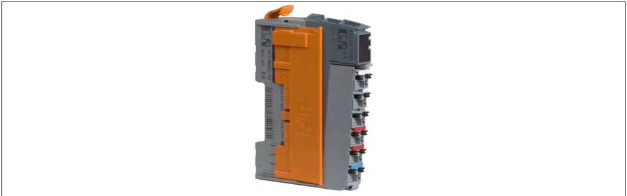
Figure 534: Lay the left locking plate on the left module and insert it in the guides
