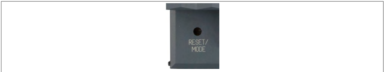
Figure 198: Reset and operating mode button
