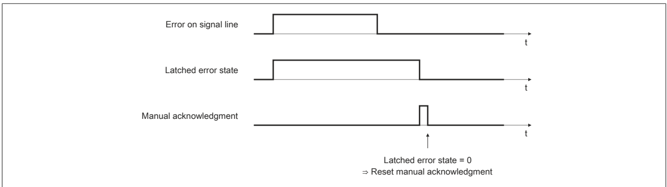
Figure 187: Cause of error corrected before being acknowledged
