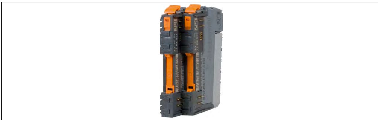
Figure 532: Connect the right module from behind to the guides for the left bus module
