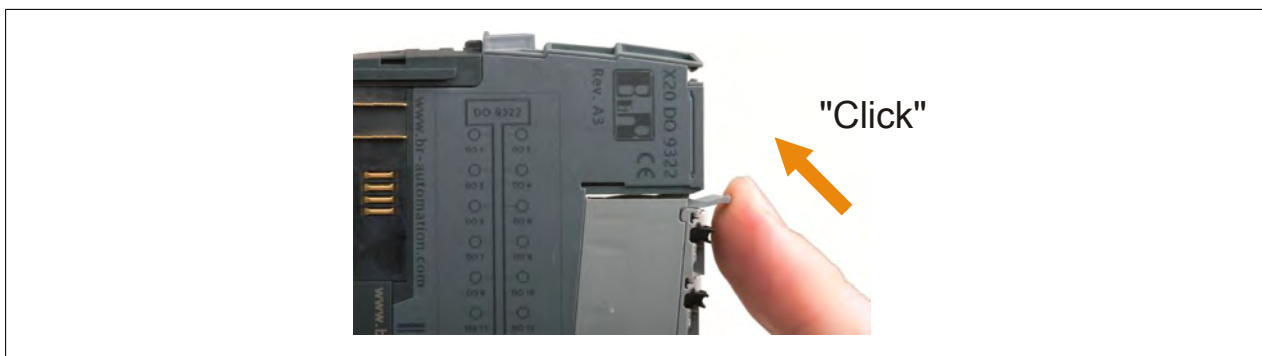
Figure 551: If the latch does not catch, the lever must be pushed up
