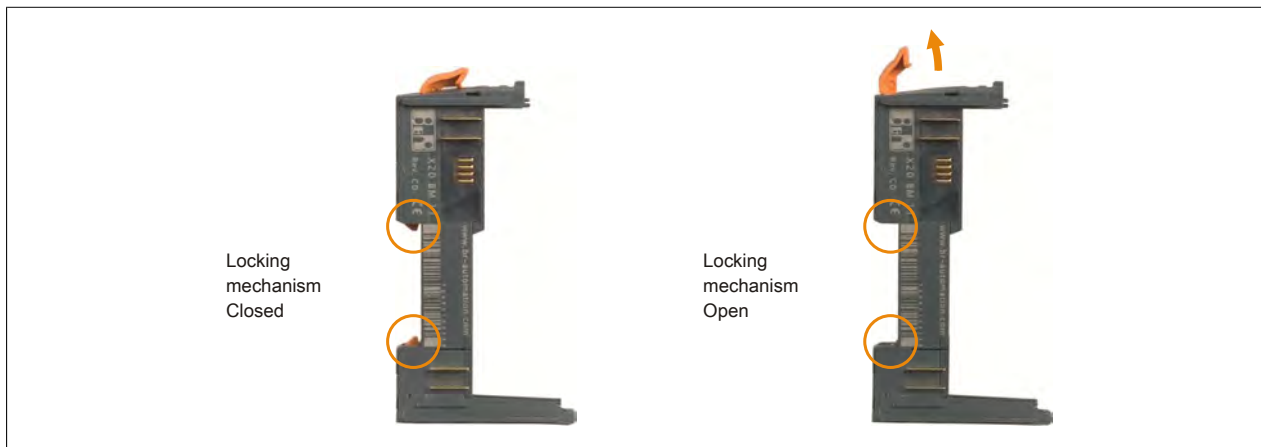
Figure 545: Push the locking lever all the way up to open the locking mechanism
